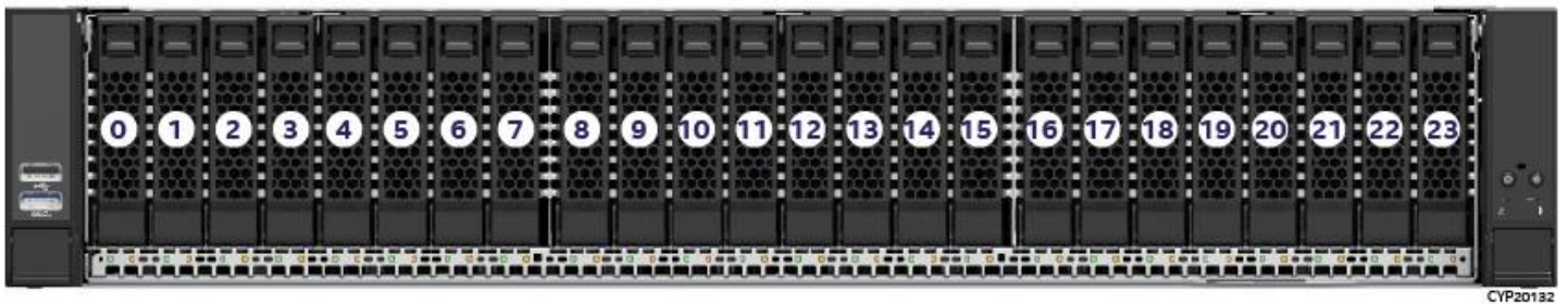
Figure 67. 24 x 2.5" Front Bay Drive Configuration (based on M50CYP2UR208)
