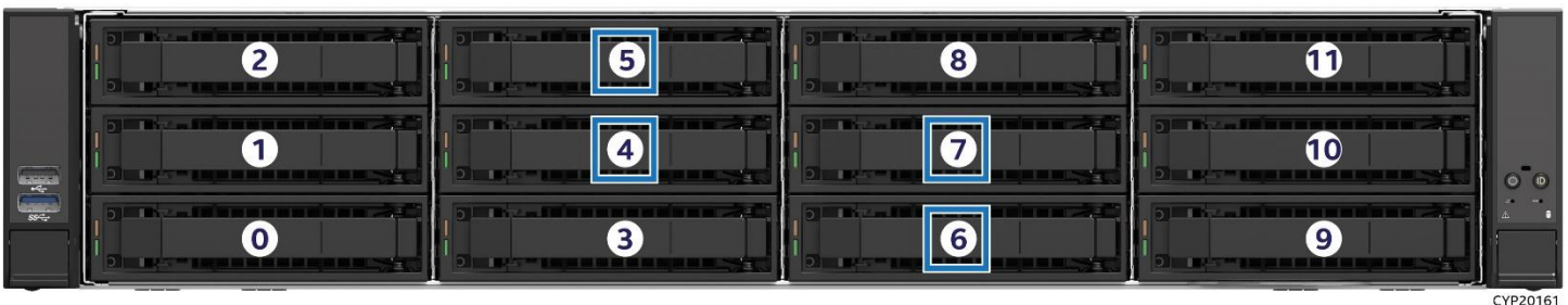
Figure 68. 12 x 3.5" Front Bay Drive Configuration – M50CYP2UR312
