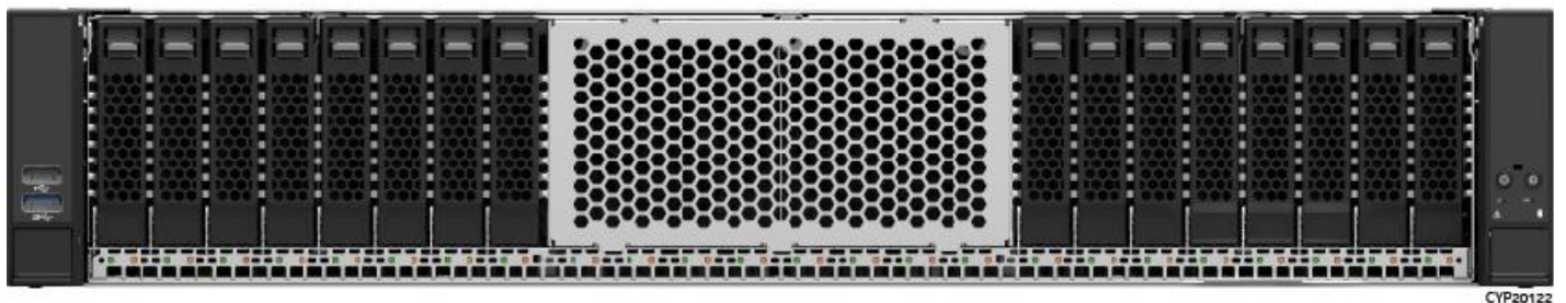
Figure 7. 16 x 2.5" Front Drive Bay Configuration (based on M50CYP2UR208)
