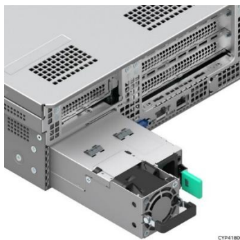
Figure 35. Power Supply Module Partially Out of Chassis
