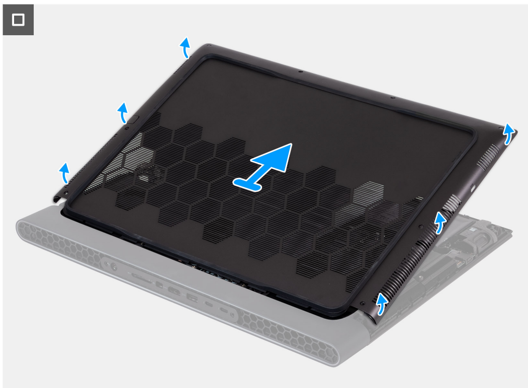
38 Figure 9 Removing the base cover Removing and installing Customer Replaceable Units (CRUs)
