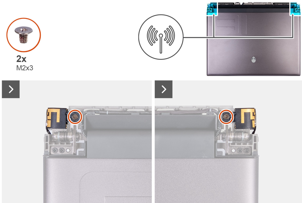
Figure 46. Removing the antenna
